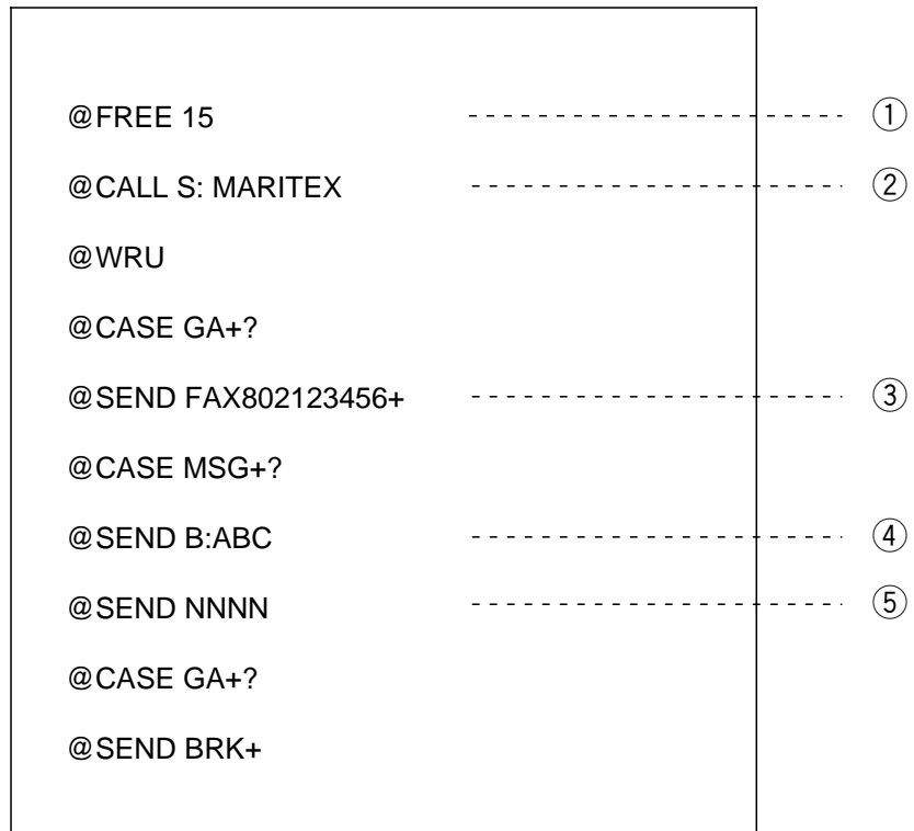
Figure 7-10 Example of macrofile for semi-fax
